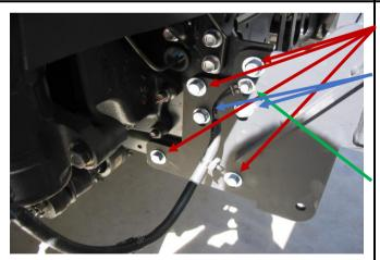
INSTALL FOUR (4) 1 ½" x ½" BOLTS, WASHERS (2 PER BOLT) AND NYLOC NUTS
