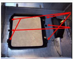
INSTALL HEADLAMP SURROUND INTO BULLBAR USING ORIGINAL FOUR (4) CLIPS
