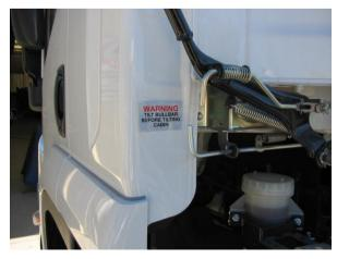
FIT TILT CAB WARNING LABEL TO BACK OF CAB NEAR TILT LEVER
