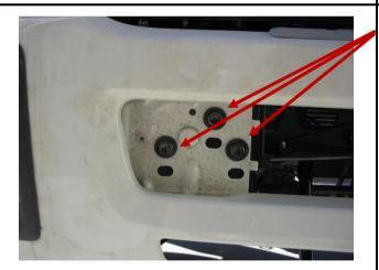
REMOVE BUMPER BOLTS, THREE (3) PER SIDE
