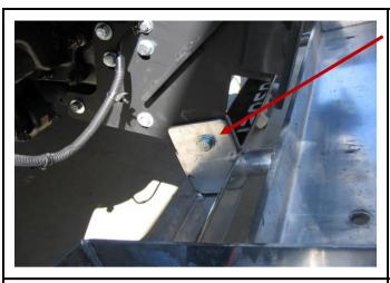
FIT BULLBAR ONTO MOUNT USING TWO (2) 2 X 5/8" BOLTS, WASHERS AND NYLOC NUT
