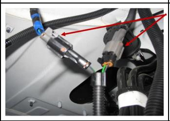
UNPLUG BODY MOUNTED INDICATOR AND PLUG BULLBAR MOUNTED INDICATOR HARNESS AS SHOWN
