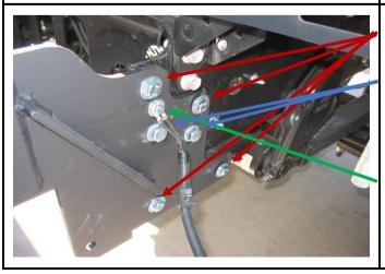
INSTALL FOUR (4) 1 ½" x ½" BOLTS, WASHERS (2 PER BOLT) AND NYLOC NUTS
