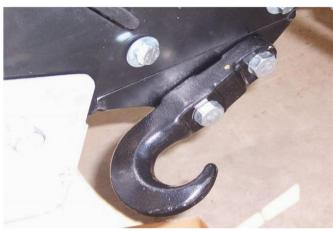
REFIT ORIGINAL TOW HOOK USING ORIGINAL BOLTS, WASHERS AND NUTS
